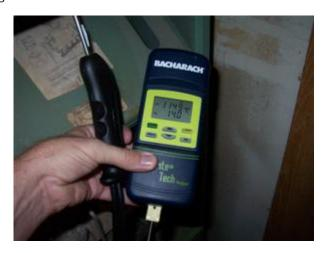
The heat exchanger had visible rusting present throughout, and the Carbon-Monoxide measured at a room heat register was approx 25 PPM. Levels above 50 PPM in the air can cause serious health issues. The furnace was recommended to be replaced, and the realtor advised the current tenants about the health risk potential. Safety is everyone's responsibility, with combustion safety a top priority for inspectors.
