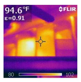
Investigation with an infra-red camera showed that the insulation along all of the upper attic knee walls was completely missing. With no insulation in these areas, all along the upper section of the home, the heat gain in summer, and heat loss in winter was tremendous.
